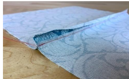
Grading of seam
